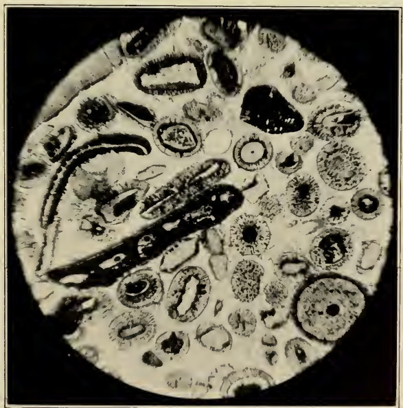
PLATE LXII.—Photomicrograph.—Dark-gray (crinoid stem) oolite, Union Limestone. x 20. (Photo. by A. Berg and W. E. Rumsey).
